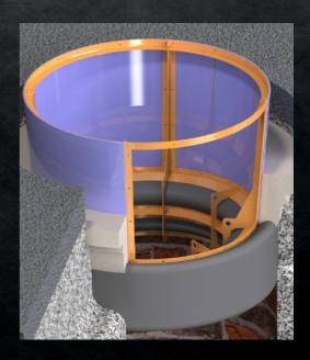
Thanks to fast and high-strength compounds, the installation of the hatch takes minimum time and traffic can be opened in 10 minutes after pouring the mixture.
